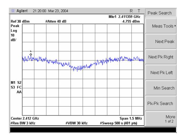
Power spectral density = -4.755dBm (< 8 dBm / 3 KHz)
