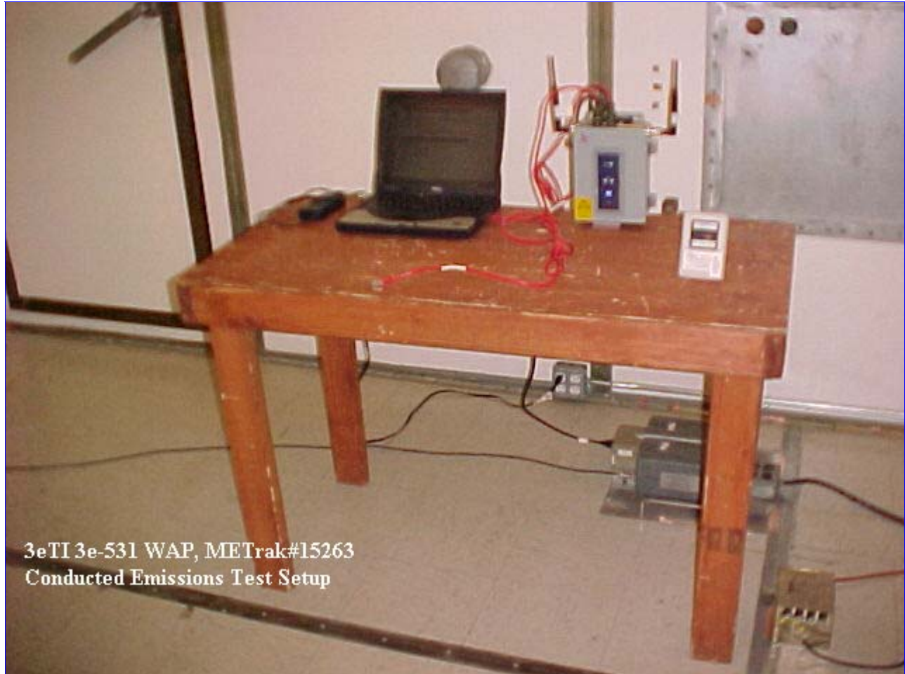
Photograph 1 Conducted Limits, Test Setup
