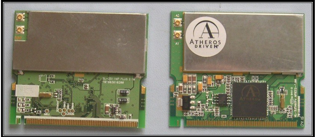
PHOTOGRAPH 11: 802.11B AND 802.11G WLAN'S FRONT VIEW
