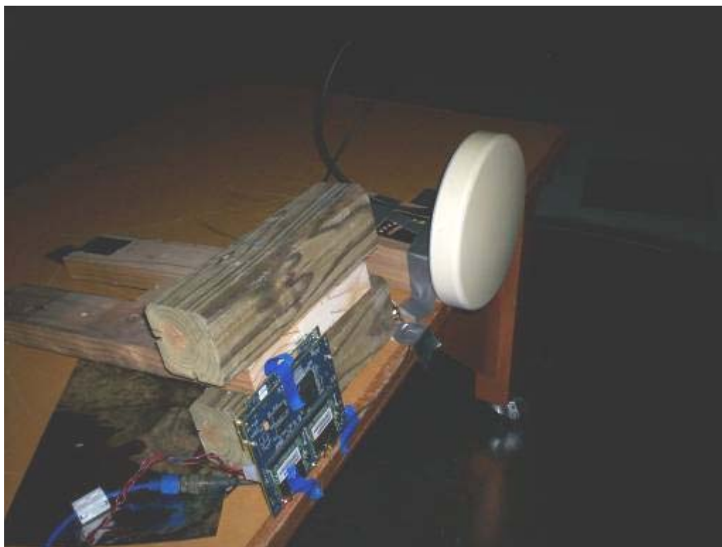
Figure 13 - EUT Test Setup, Vertical Orientation, HG5817D
