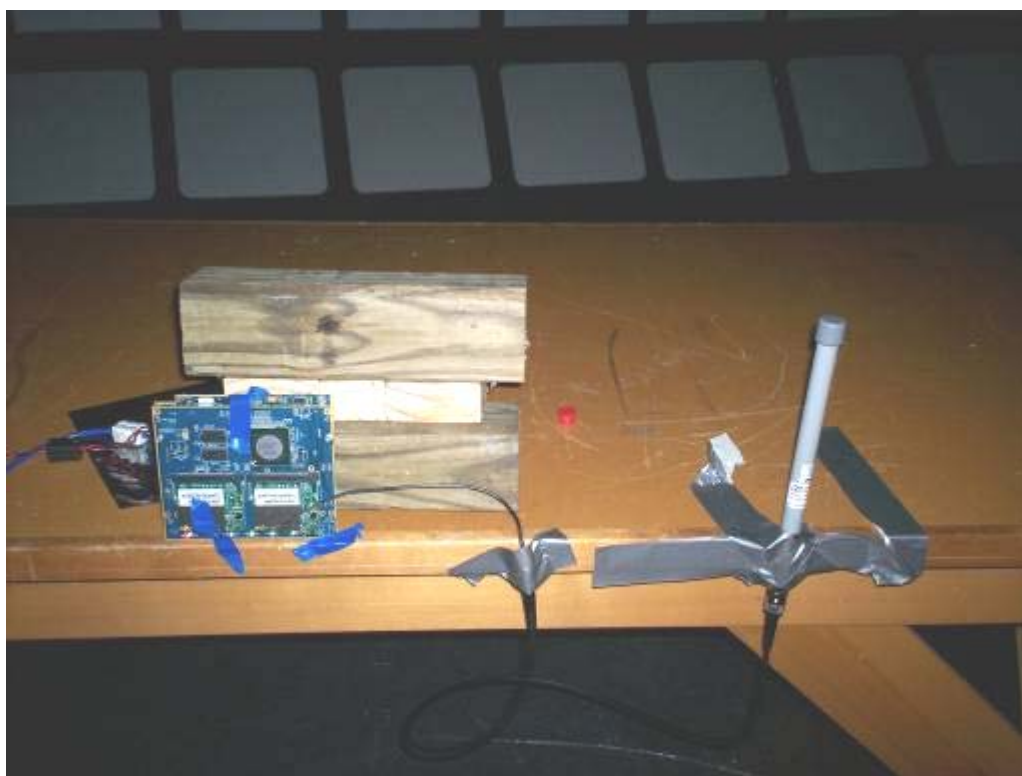
Figure 14 - EUT Test Setup, Vertical Orientation, HG5808U
