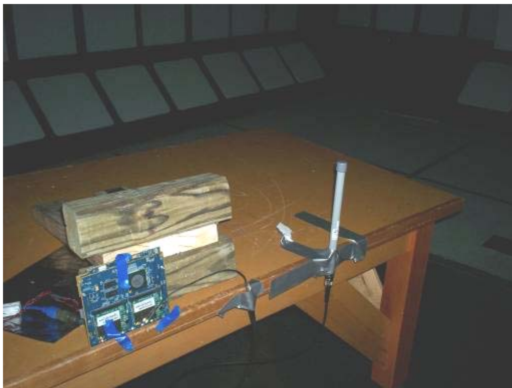
Figure 15 - EUT Test Setup, Vertical Orientation, HG5808U
