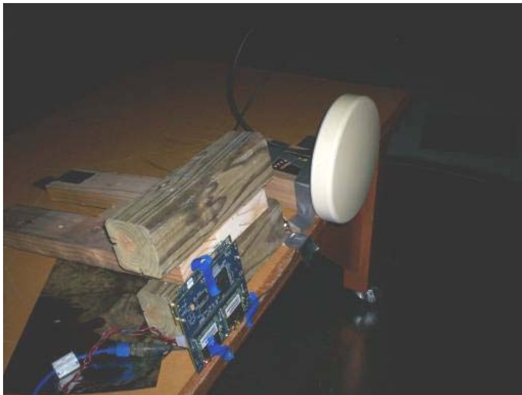
Figure 56 - EUT Test Setup, Vertical Orientation, HG5817D
