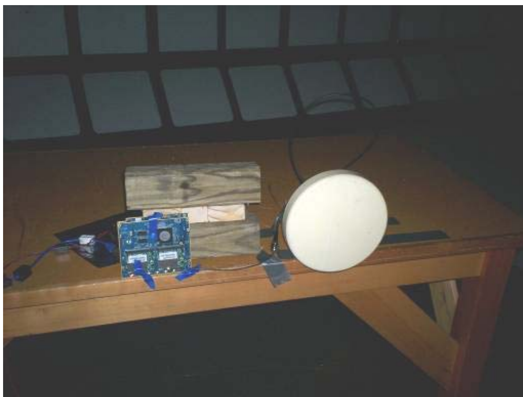
Figure 55 - EUT Test Setup, Vertical Orientation, HG5817D
