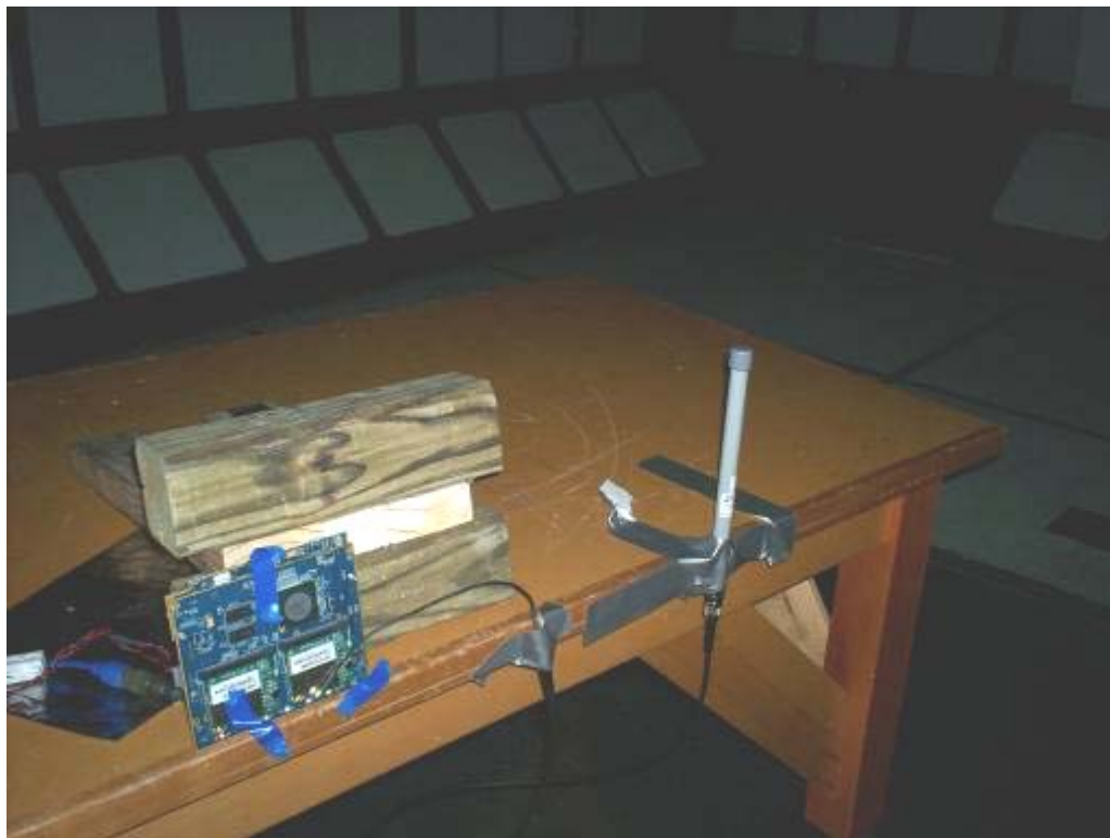
Figure 58 - EUT Test Setup, Vertical Orientation, HG5808U
