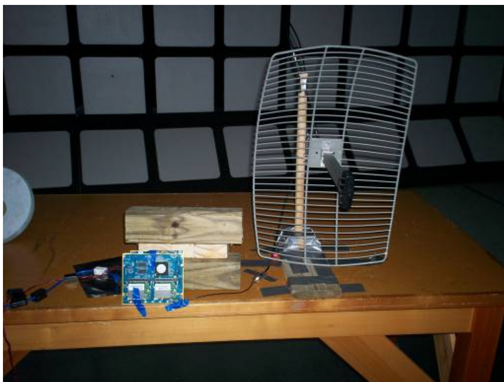
Figure 53 - EUT Test Setup, Vertical Orientation, HG2424G
