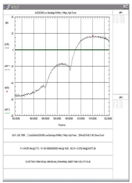
Figure 22: Lower Band-edge, 11Mbps, High Power
