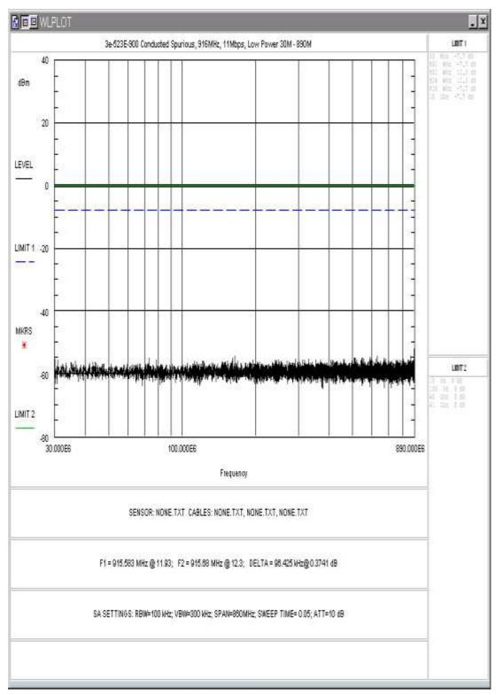
Figure 17: Conducted Spurious Emissions, 11Mbps, Low Power, 30 - 890MHz
