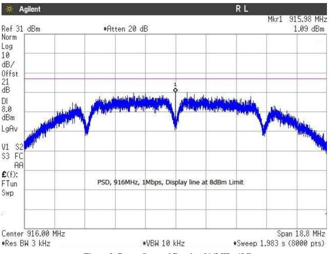
Figure 3: Power Spectral Density, 916MHz, 1Mbps
