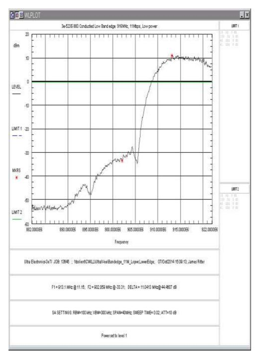
Figure 24: Lower Band-edge, 11Mbps, Low Power
