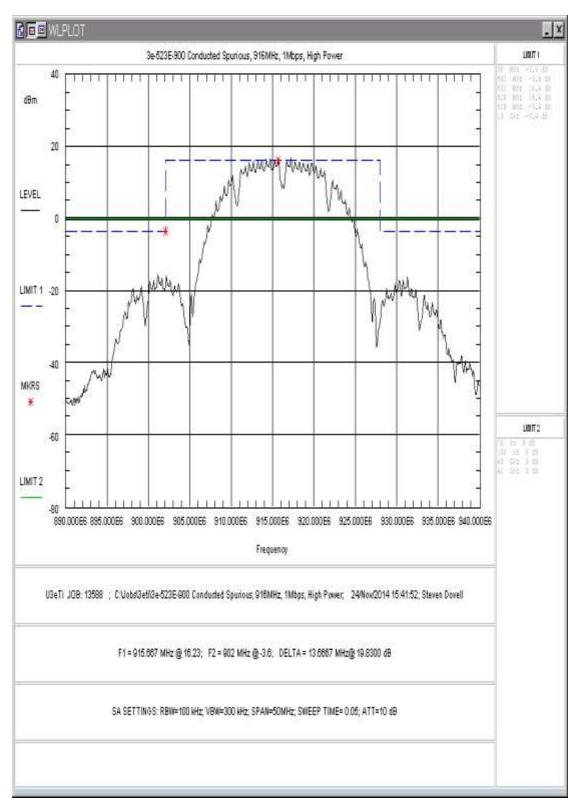
Figure 6: Conducted Spurious Emissions, 1Mbps, High Power, 890 -940MHz
