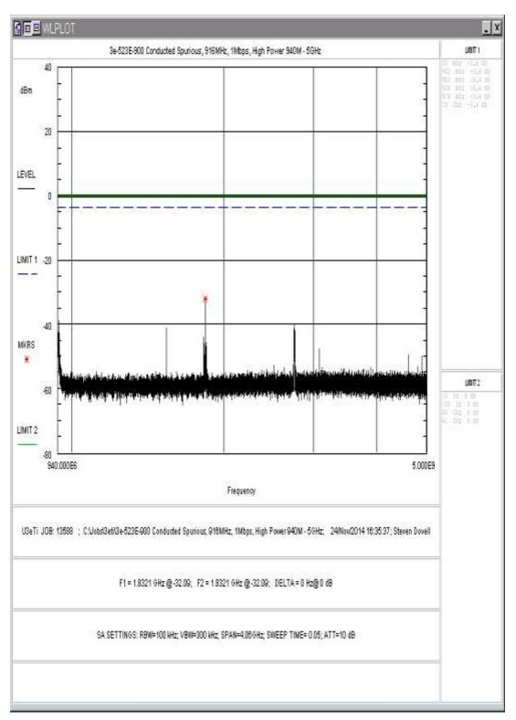
Figure 7: Conducted Spurious Emissions, 1Mbps, High Power, 940 – 5000MHz
