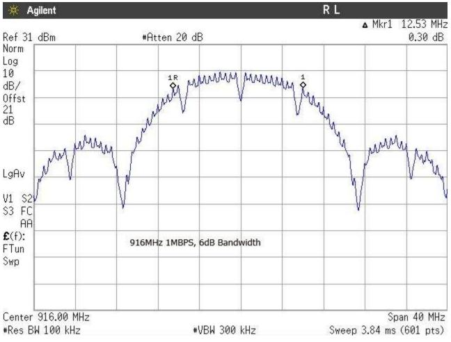
Figure 1: Occupied Bandwidth, 916MHz, 1Mbps
