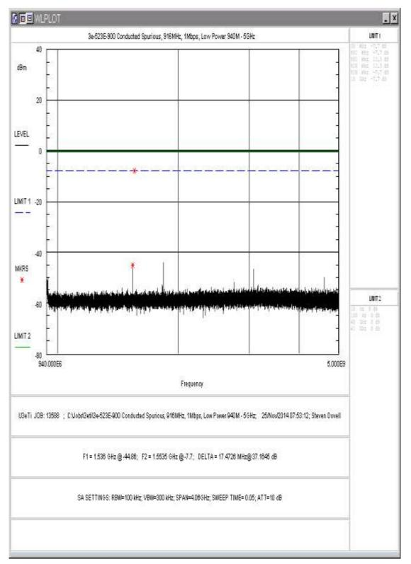
Figure 15: Conducted Spurious Emissions, 1Mbps, Low Power, 940-5000MHz
