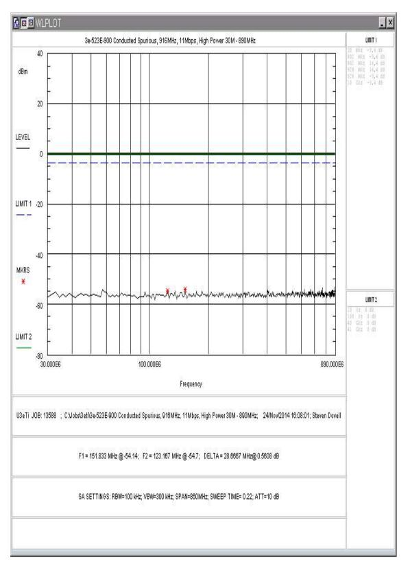
Figure 9: Conducted Spurious Emissions, 11Mbps, High Power, 30 - 890MHz
