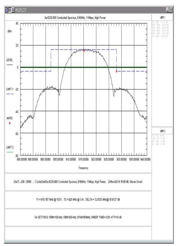
Figure 10: Conducted Spurious Emissions, 11Mbps, High Power, 890-940MHz
