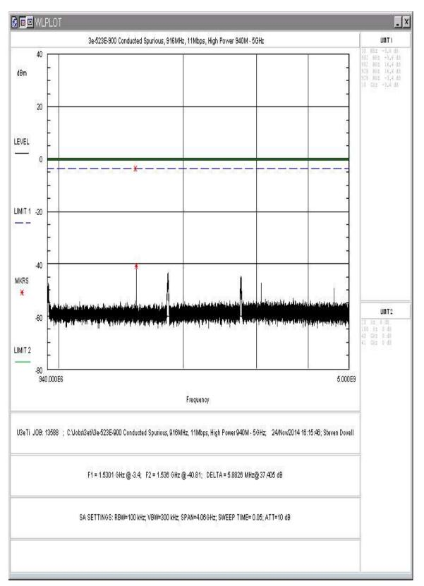
Figure 11: Conducted Spurious Emissions, 11Mbps, High Power, 940-5000MHz
