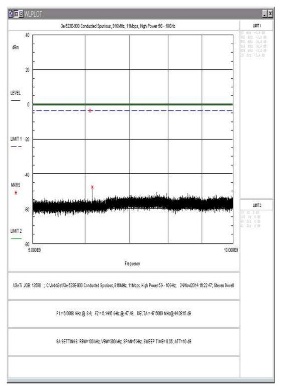
Figure 12: Conducted Spurious Emissions, 11Mbps, High Power, 5-10GHz
