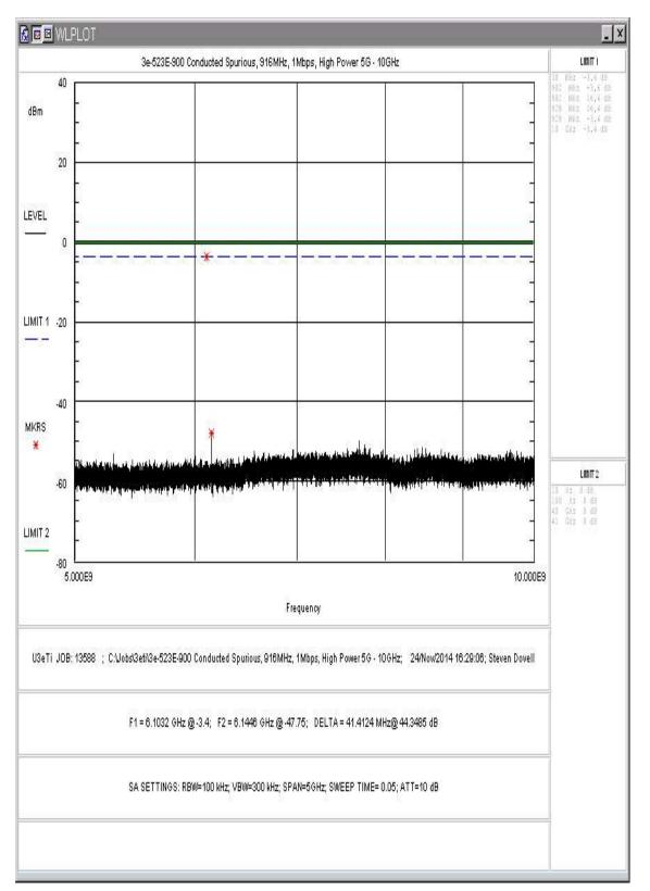
Figure 8: Conducted Spurious Emissions, 1Mbps, High Power, 5 - 10GHz
