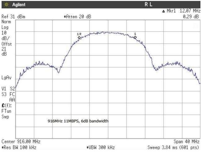
Figure 2: Occupied Bandwidth, 916MHz, 11Mbps
