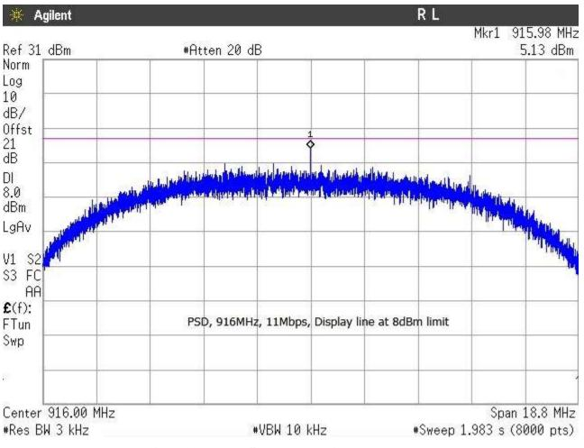
Figure 4: Power Spectral Density, 916MHz, 11Mbps
