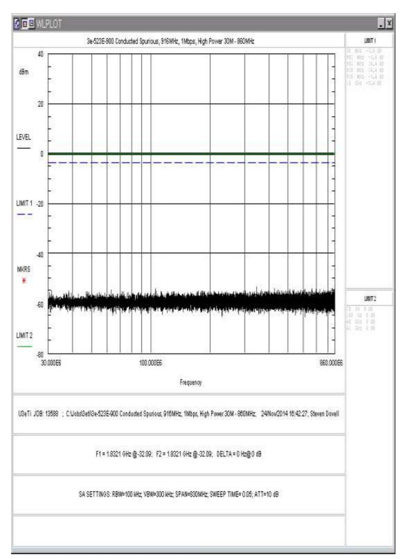
Figure 5: Conducted Spurious Emissions, 1Mbps, High Power, 30 - 890MHz
