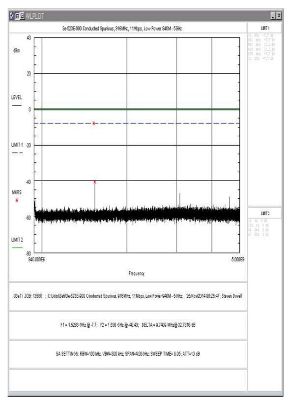
Figure 19: Conducted Spurious Emissions, 11Mbps, Low Power, 940-5000MHz
