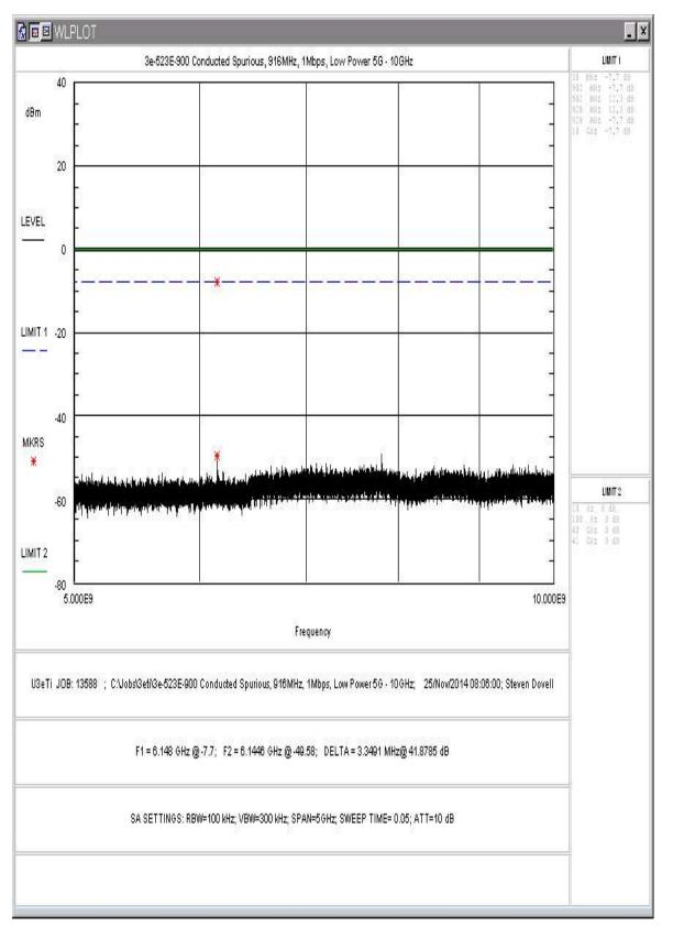
Figure 16: Conducted Spurious Emissions, 1Mbps, Low Power, 5-10GHz
