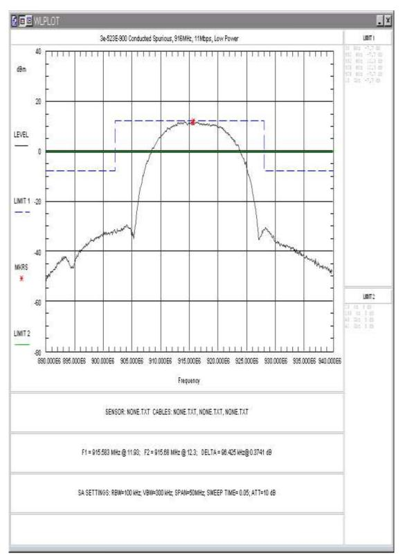
Figure 18: Conducted Spurious Emissions, 11Mbps, Low Power, 890-940MHz
