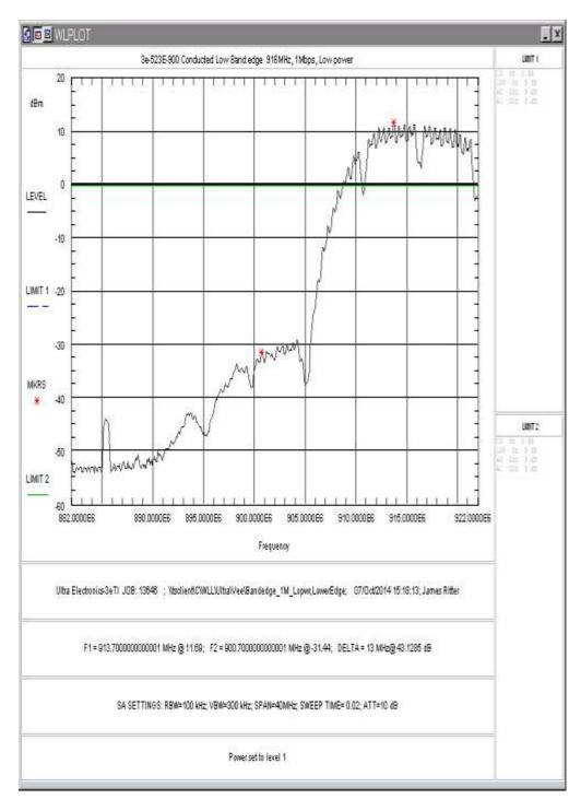
Figure 23: Lower Band-edge, 1Mbps, Low Power
