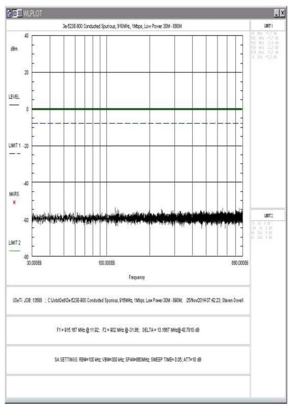
Figure 13: Conducted Spurious Emissions, 1Mbps, Low Power, 30 - 890MHz
