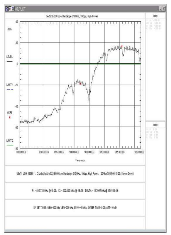
Figure 21: Lower Band-edge, 1Mbps, High Power
