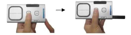
When the Bluetooth Indicator turns blinking red/blue, release the Accept Button. This means the kit is now in pairing mode.
