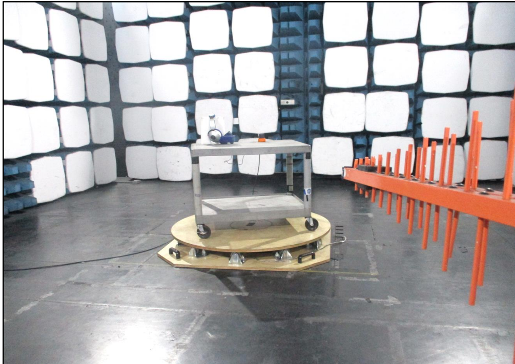
Figure 20 - Test Setup - 30 MHz to 1 GHz - Y Orientation
