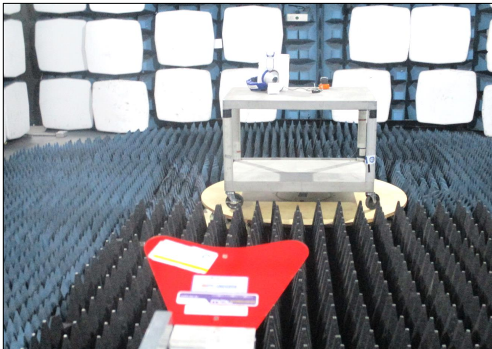
Figure 21 - Test Setup - 1 GHz to 13 GHz - Y Orientation
