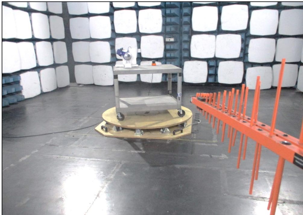
Figure 28 - Test Setup - 30 MHz to 1 GHz - Z Orientation
