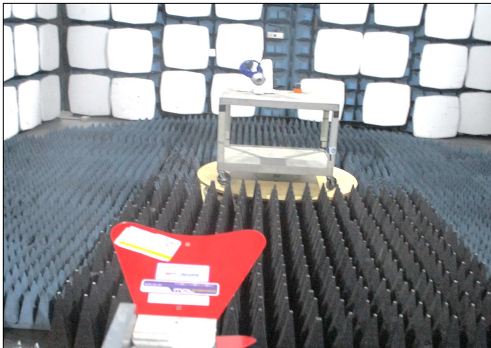
Figure 29 - Test Setup - 1 GHz to 13 GHz - Z Orientation
