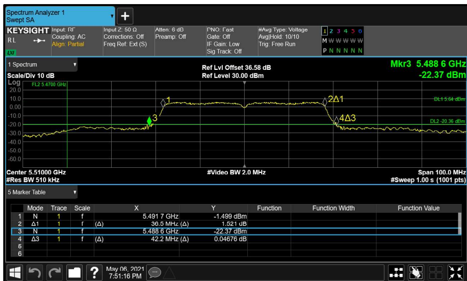
Figure 142 - Aux (B) 5510 MHz (CH102) 26 dB and 99% Bandwidth
