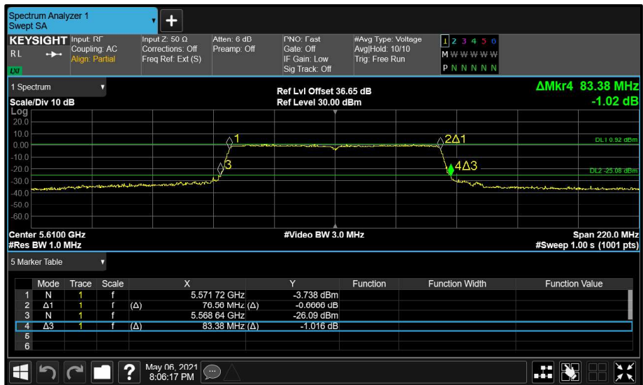
Figure 166 - Aux (B) 5610 MHz (CH122) 26 dB and 99% Bandwidth
