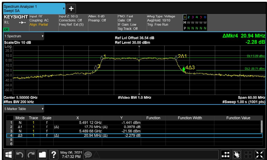
Figure 126 - Aux (B) 5500 MHz (CH100) 26 dB and 99% Bandwidth
