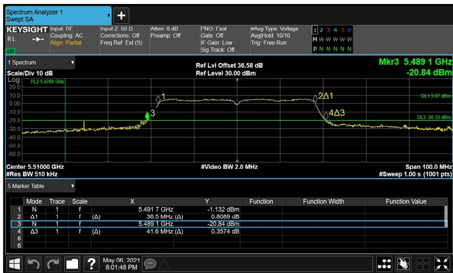
Figure 150 - Aux (B) 5510 MHz (CH102) 26 dB and 99% Bandwidth
