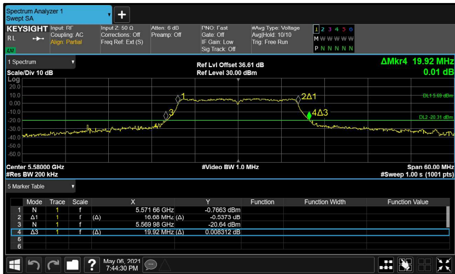
Figure 120 - Aux (B) 5580 MHz (CH116) 26 dB and 99% Bandwidth
