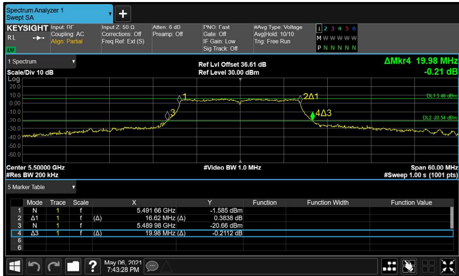
Figure 117 - Main (A) 5500 MHz (CH100) 26 dB and 99% Bandwidth
