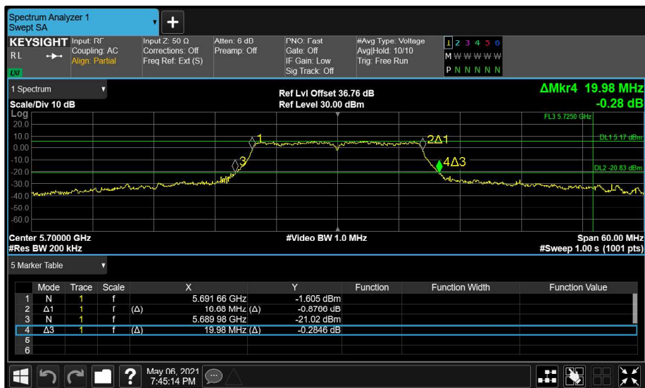
Figure 122 - Aux (B) 5700 MHz (CH140) 26 dB and 99% Bandwidth
