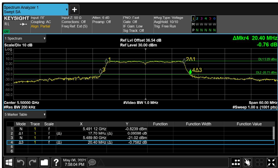
Figure 134 - Aux (B) 5500 MHz (CH100) 26 dB and 99% Bandwidth
