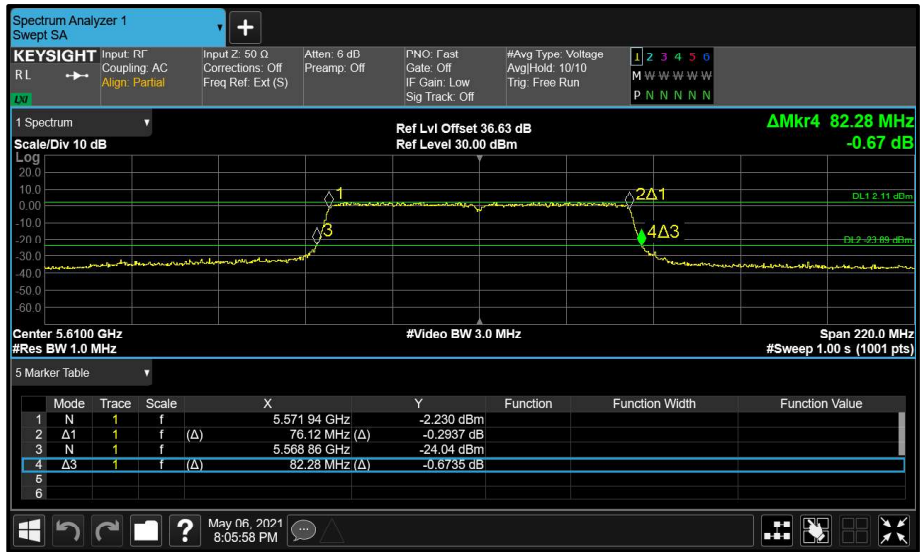
Figure 165 - Main (A) 5610 MHz (CH122) 26 dB and 99% Bandwidth
