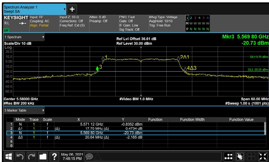
Figure 128 - Aux (B) 5580 MHz (CH116) 26 dB and 99% Bandwidth
