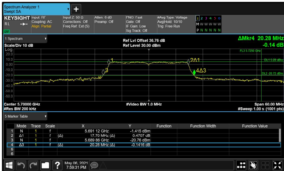
Figure 138 - Aux (B) 5700 MHz (CH140) 26 dB and 99% Bandwidth
