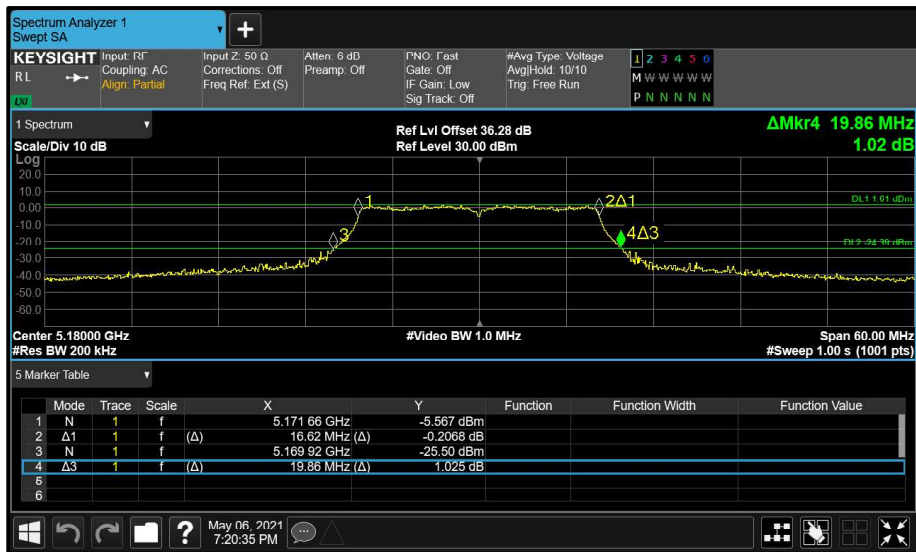
Figure 33 - Main (A) 5180 MHz (CH36) 26 dB and 99% Bandwidth
