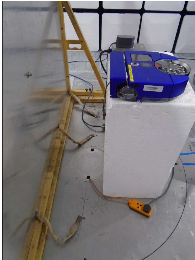
Figure 144 - Test Setup - AC Line Conducted Emissions
