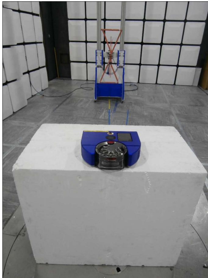
Figure 146 - Test Setup - 30 MHz to 1 GHz
