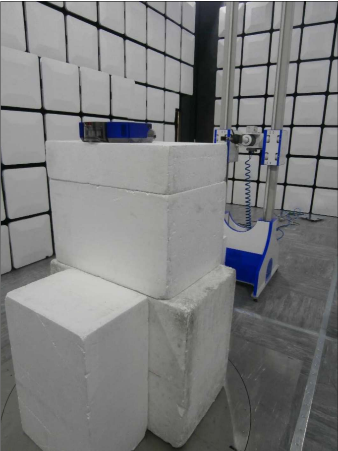
Figure 148 - Test Setup - 18 GHz to 25 GHz
