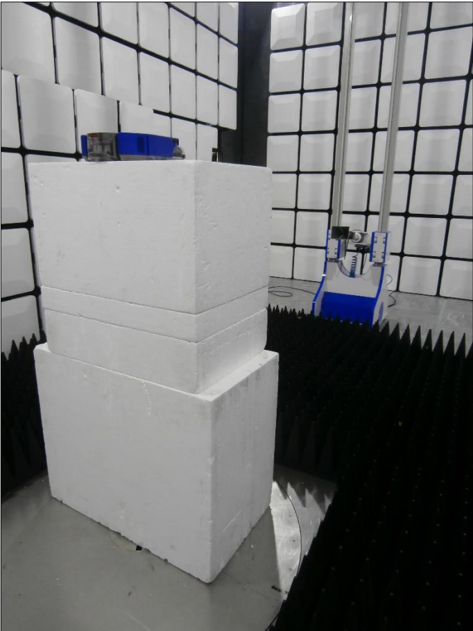
Figure 31 - Test Setup - 1 GHz to 18 GHz
