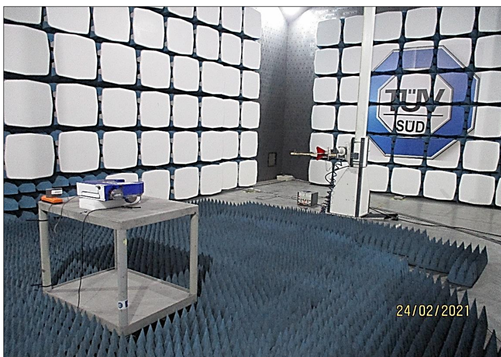
Figure 2 - Test Setup - 1 GHz to 18 GHz
