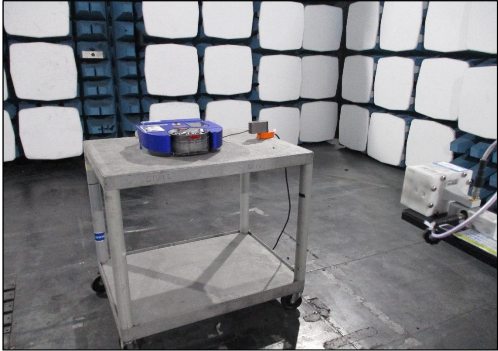
Figure 3 - Test Setup - 18 GHz to 30 GHz
