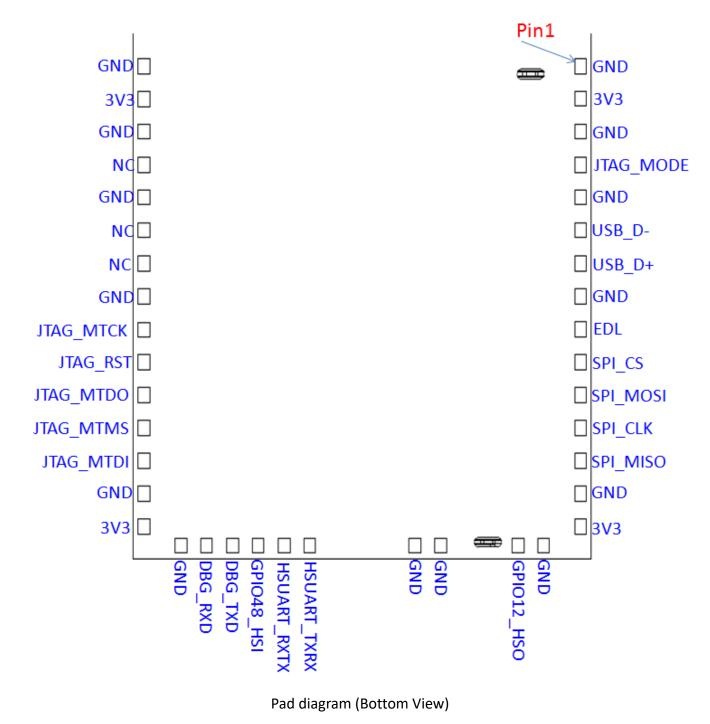
There are Gnd Pads for thermal purpose on the bottom but not shown here, please refer detailed land pattern in section 5.2.
