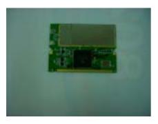
GL2422MP, the wireless Ethernet adapter for mini PCI type IIIB compliant notebook PCs, set-top box and integrated device, is fully compatible with IEEE 802.11b standard and supporting higher data rate to 22Mbps. Using Direct Sequence spread spectrum technology for immunity from interference, it will automatically fallback to lower data rate in the environment of interference.
