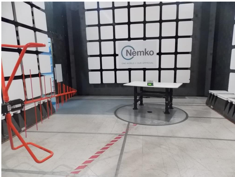
Figure 1-2: Radiated emissions setup photo
