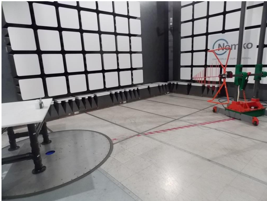
Figure 1-1: Radiated emissions setup photo
