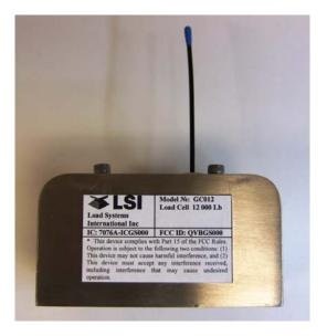
The label is installed on the transmitter box, centered on the long side of the box for all products.
