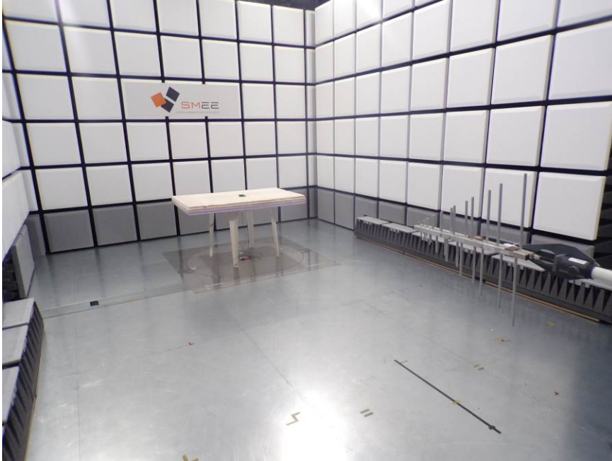
Test setup for frequency below 1GHz
