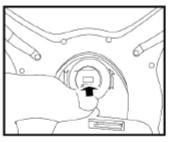
1.Insert the camera's connector wire into the interface on the main body.
