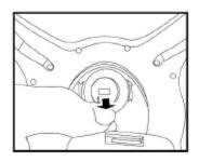
2.Then taking out the camera upward and pulling out the connector
