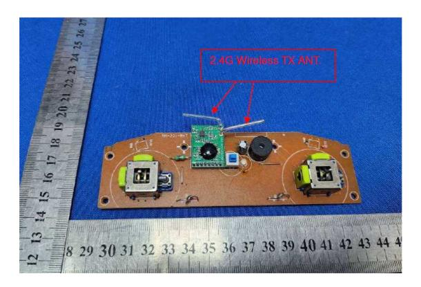
Antenna Type: Wire Antenna
