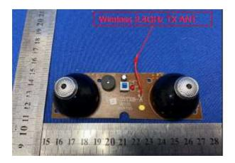
Antenna Type: Wire Antenna
