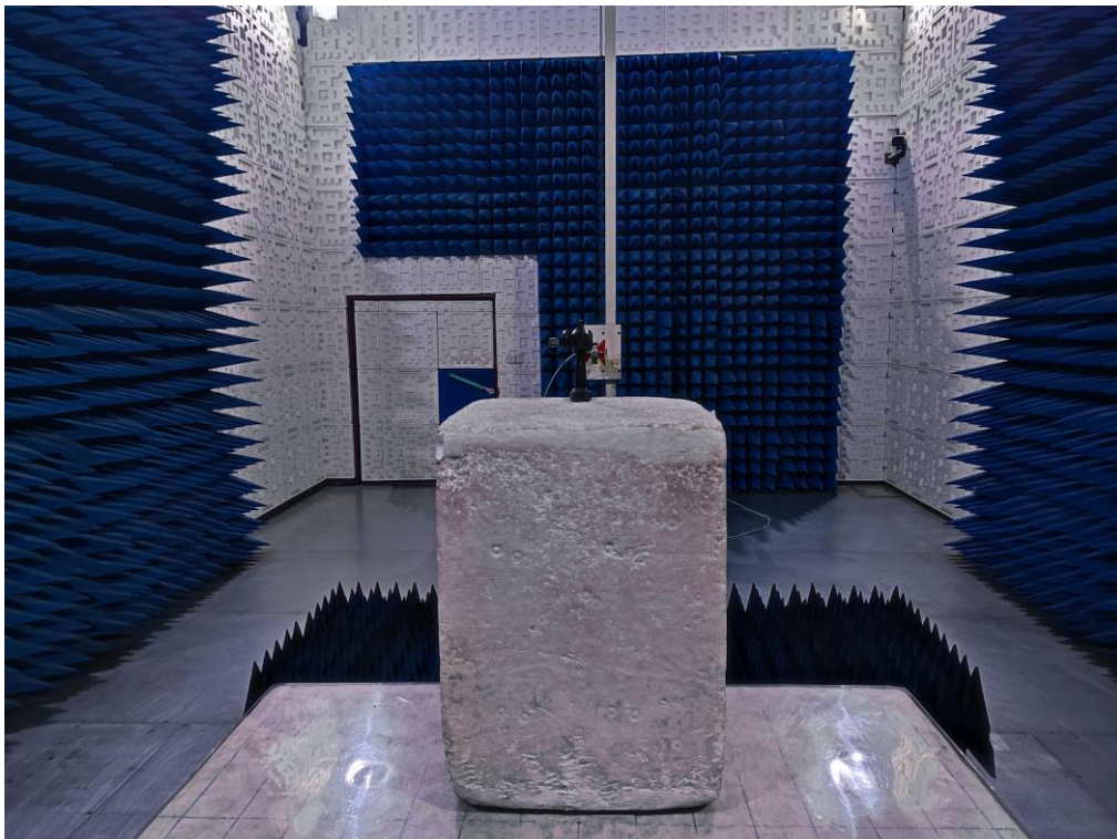
RADIATED EMISSION TEST SETUP ABOVE 1GHz
