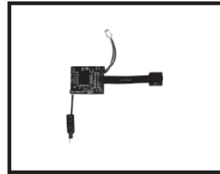
Camera circuit board
