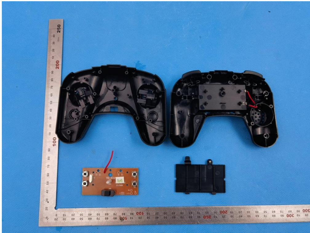
INTERNAL VIEW OF EUT (FIGURE 1)
