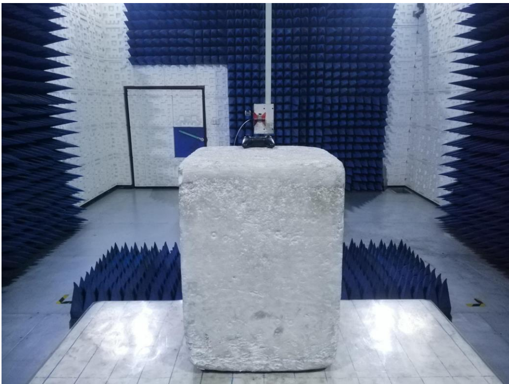
RADIATED EMISSION TEST SETUP ABOVE 1GHz
