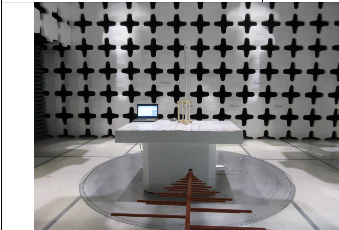
Radiated Emission Test below 1GHz Rear View- Dipole Antenna
