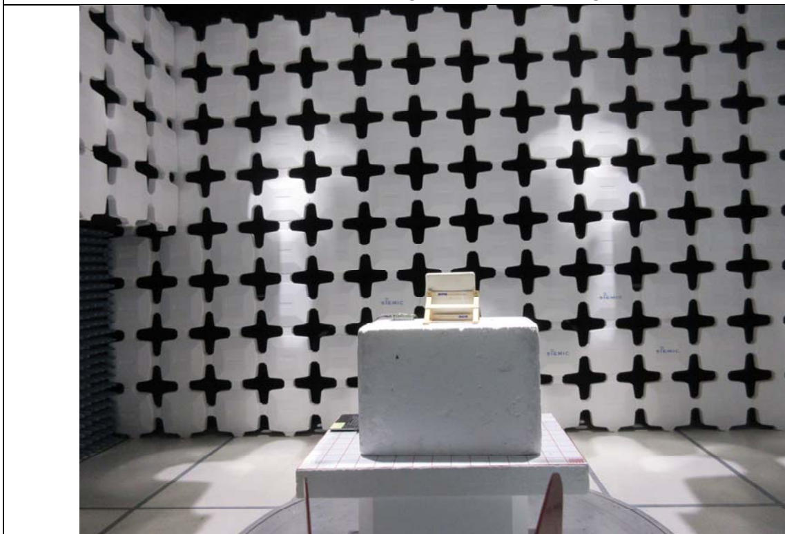
Radiated Emission Test above 1GHz Rear View- RHCP Patch Antenna
