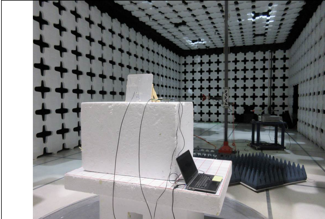
Radiated Emission Test above 1GHz Front View- RHCP Patch Antenna
