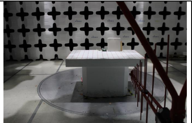
Radiated Emission Below 1G – Rear View
