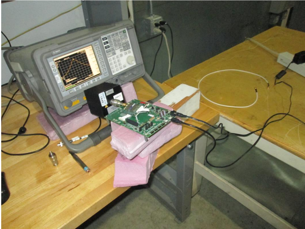
Conducted EMI Testing at the Antenna port
