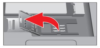
4. Insert the SIM card into the holder. Make sure the golden contacts face the socket.
