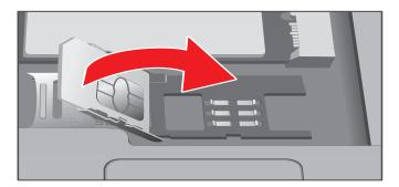
6. Slide the SIM card holder to the "LOCK" direction.
