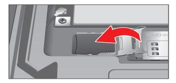
6. Slide the microSD socket cover to the "LOCK" direction.
