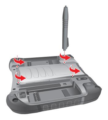
CAUTION: Avoid damaging the cable connectors. RS-232 and USB cables are connected to the motherboard under the compartment cover.
