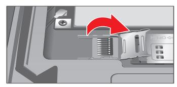
4. Place the microSD card into the socket, connectors facing the golden socket connectors.
