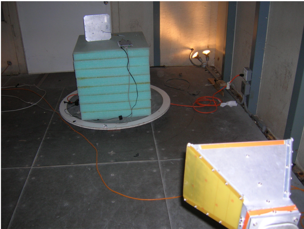
Radiated Emissions Setup
