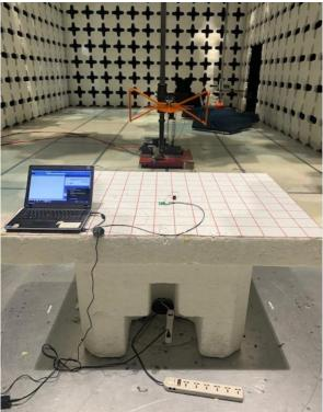
Radiated Emission Test below 1GHz Rear View
