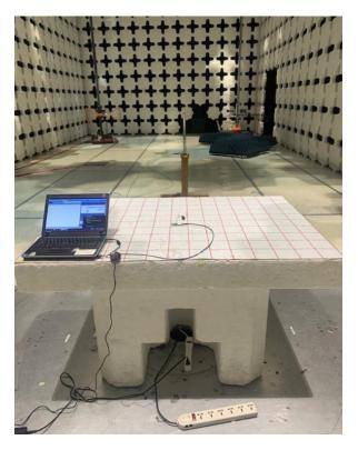
Radiated Emission Test below 30MHz Rear View
