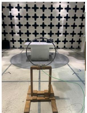
Radiated Emission Test below 30MHz Front View
