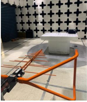
Radiated Emission Test below 1GHz Front View
