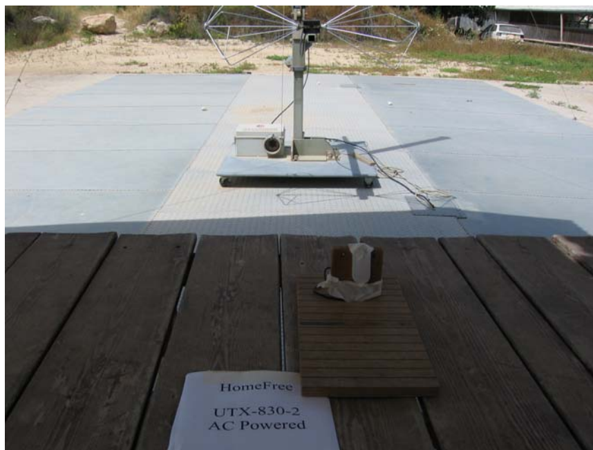
Figure 5. Radiated Emission Test 30 - 1000MHz
