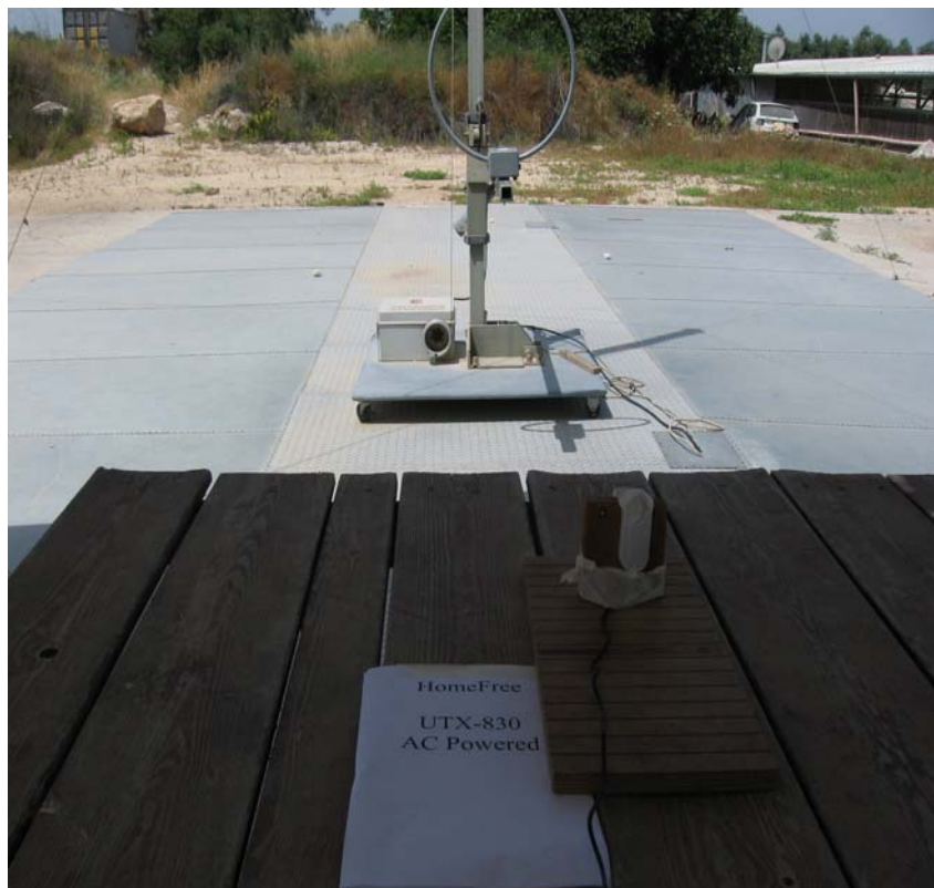
Figure 4. Radiated Emission Test 9 kHz – 30 MHz
