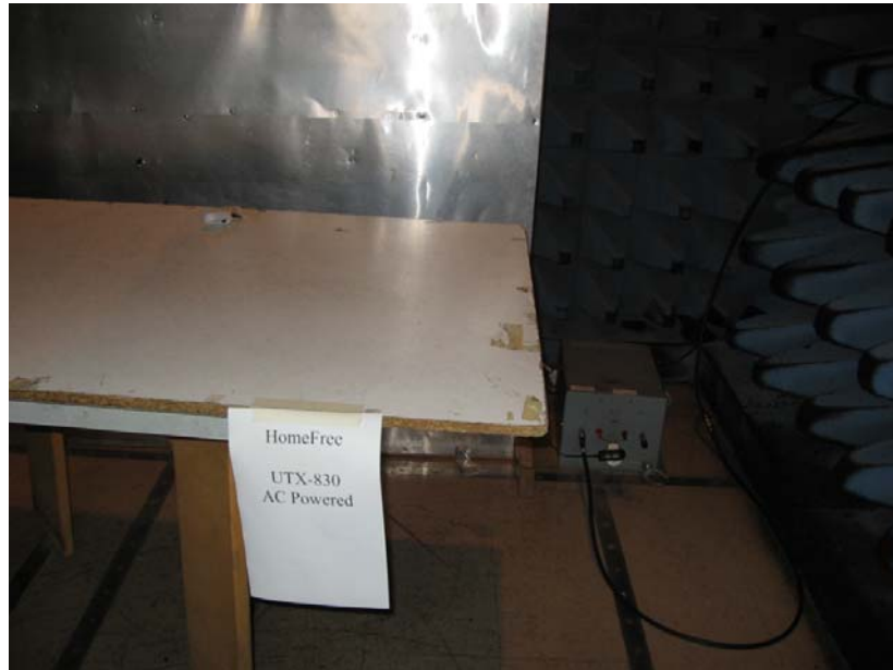
Figure 2. Conducted Emission Test
