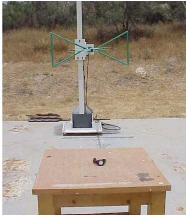
Photo 2. Spurious emissions test setup.
