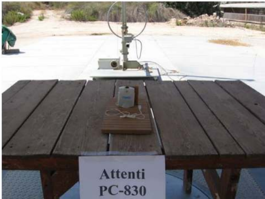
Figure 2. Radiated Emission Test 9 kHz – 30 MHz
