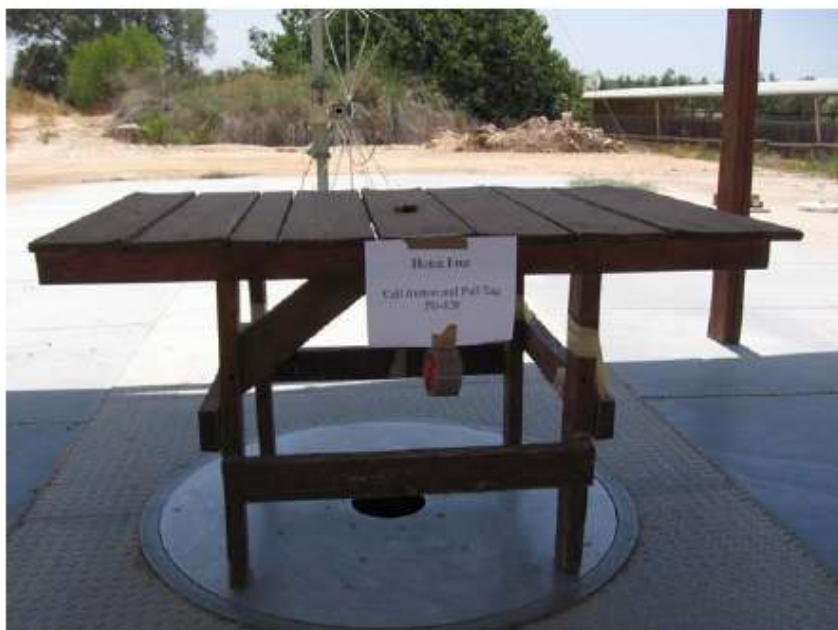
Figure 3. Radiated Emission Test 30 MHz – 3200 MHz
