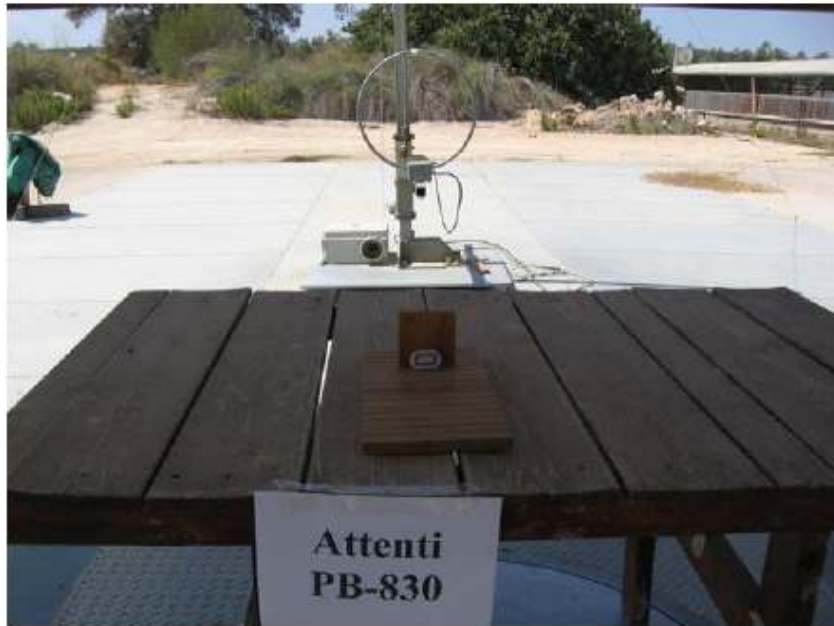
Figure 2. Radiated Emission Test 9 kHz – 30 MHz
