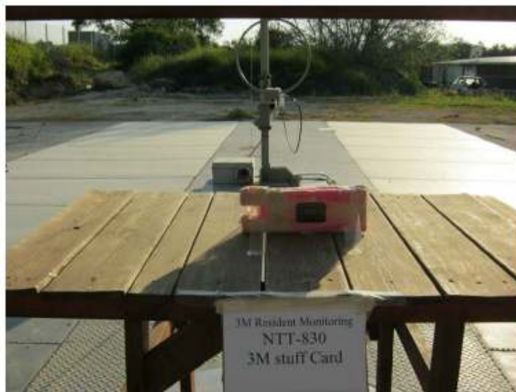
Figure 2. Radiated Emission Test 9 kHz – 30 MHz
