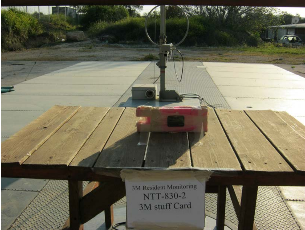
Figure 2. Radiated Emission Test 9KHz-30MHz
