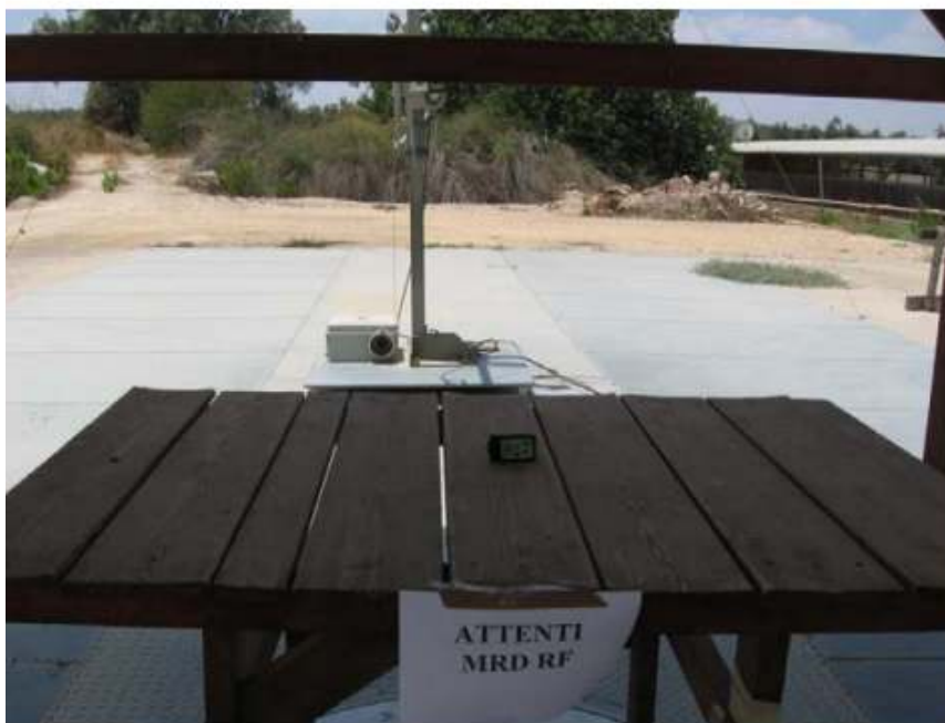
Figure 3. Radiated Emission Test 30 – 4500 MHz
