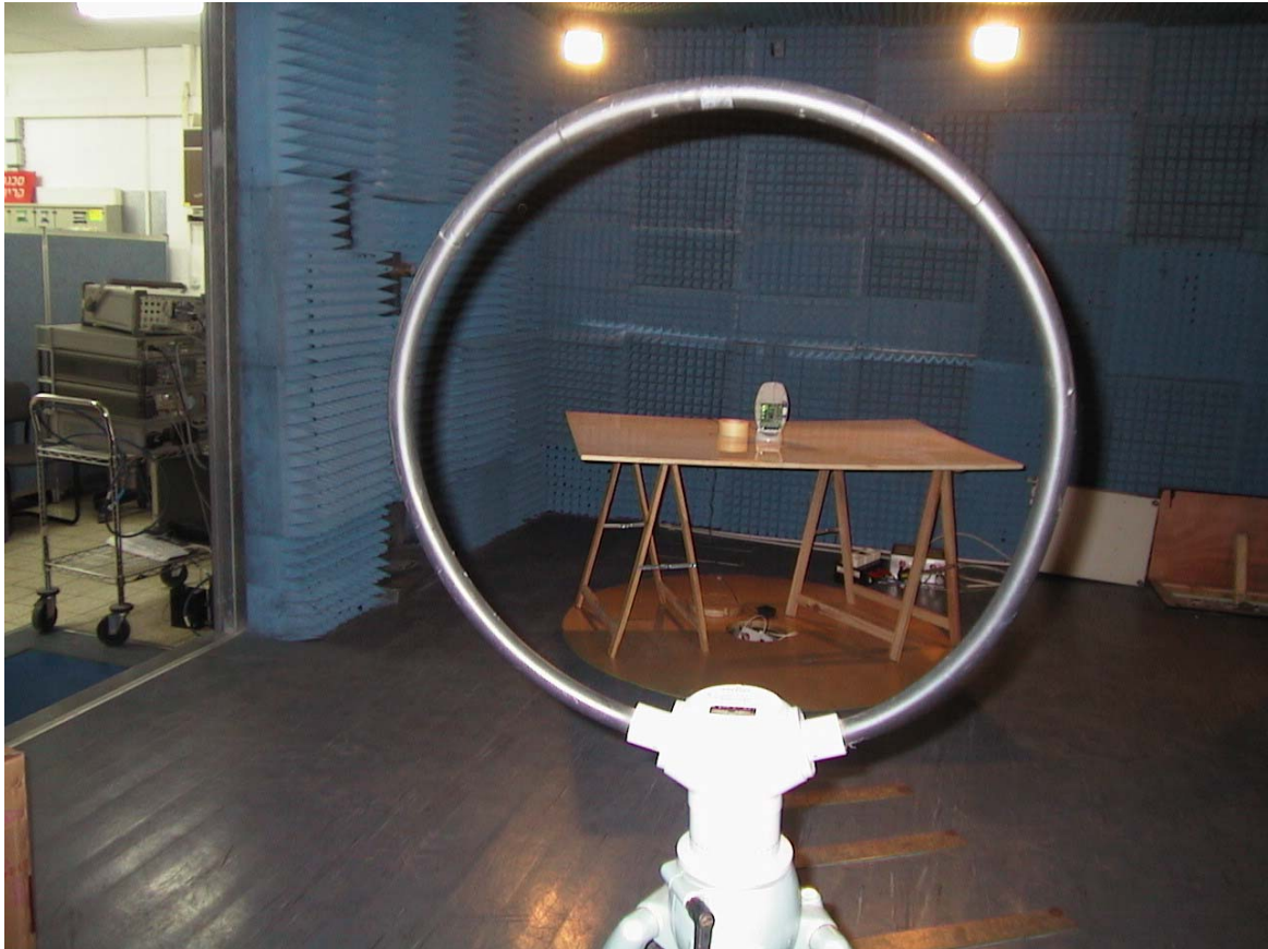
Radiated Emission Test Setup up to 30MHz
