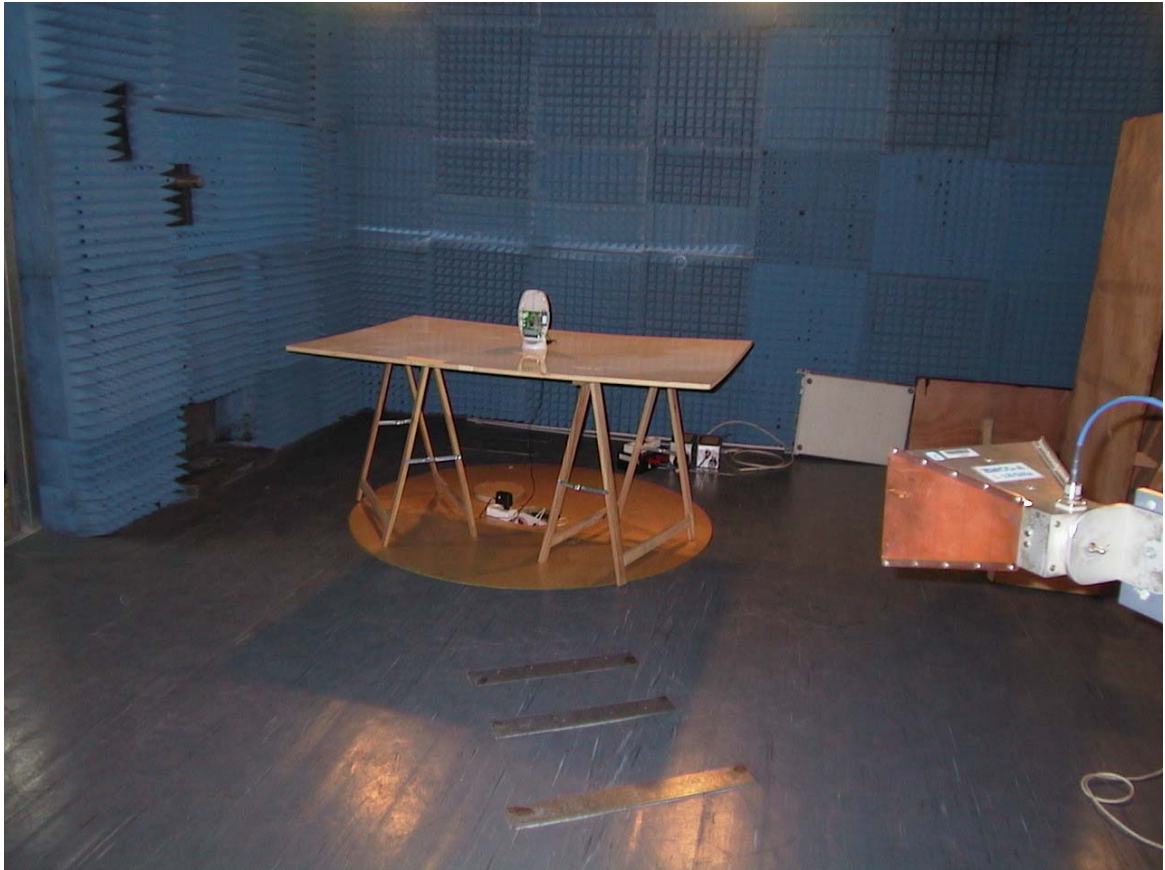
Radiated Emission Test Setup 1GHz-18GHz
