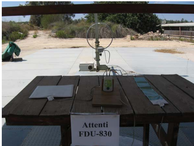
Figure 2. Radiated Emission Test 9 kHz – 30 MHz
