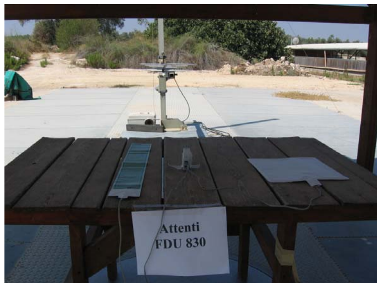
Figure 3. Radiated Emission Test 30 – 4500 MHz
