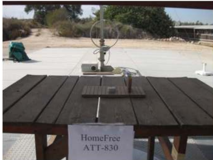
Figure 2. Radiated Emission Test 9 kHz – 30 MHz
