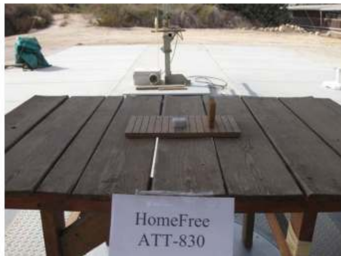
Figure 3. Radiated Emission Test 30 MHz- 3.5 GHz
