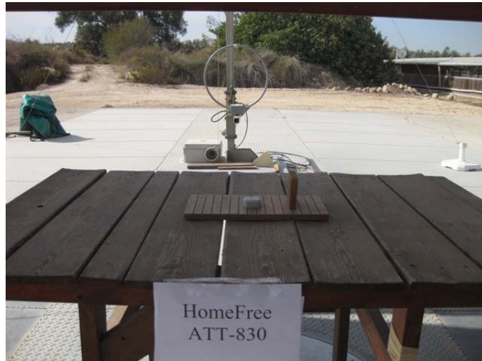
Figure 2. Radiated Emission Test 9 kHz – 30 MHz
