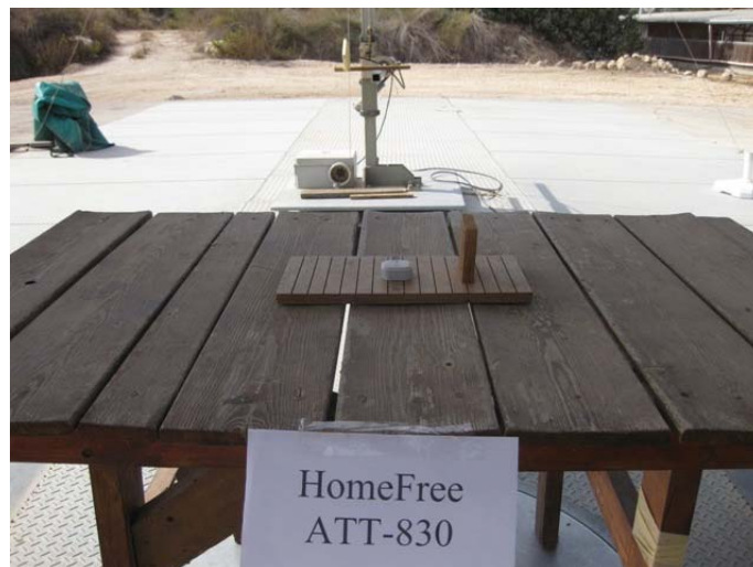
Figure 3. Radiated Emission Test 30 MHz- 3.5 GHz
