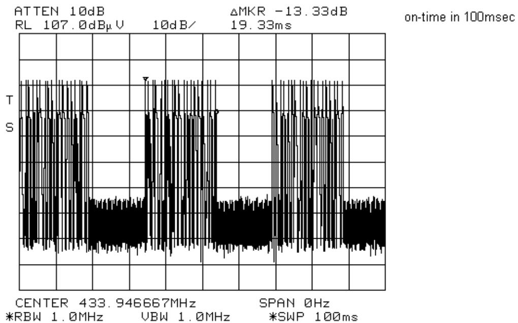
Duty cycle correction =  $20\log((19.33 \times 3)/100) = -4.7\text{dB}$
