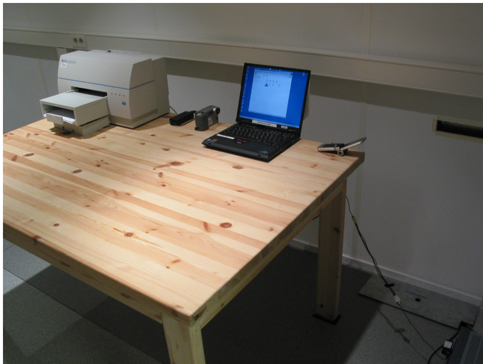
Picture 3 AC powerline conducted emission measurement
