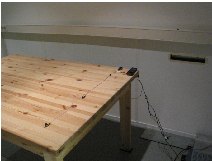
Picture 4 AC powerline conducted emission measurement Bluetooth TX / WLAN TX / FM TX
