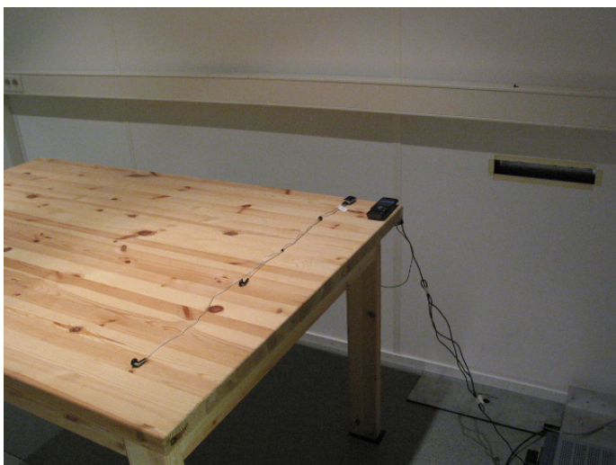
Picture 4 AC powerline conducted emission measurement Bluetooth TX / WLAN TX / FM TX
