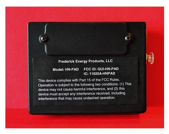
Material: Avery 2920 Clear Overlaminate (Gloss – 4 yr film) Final Thickness 0.006 – 0.010" Permanent Adhesion Labels will be pre-cut to size
