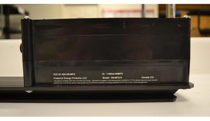
Material: Avery 2920 Clear Overlaminate (Gloss – 4 yr film) Final Thickness 0.006 – 0.010" Permanent Adhesion Labels will be pre-cut to size
