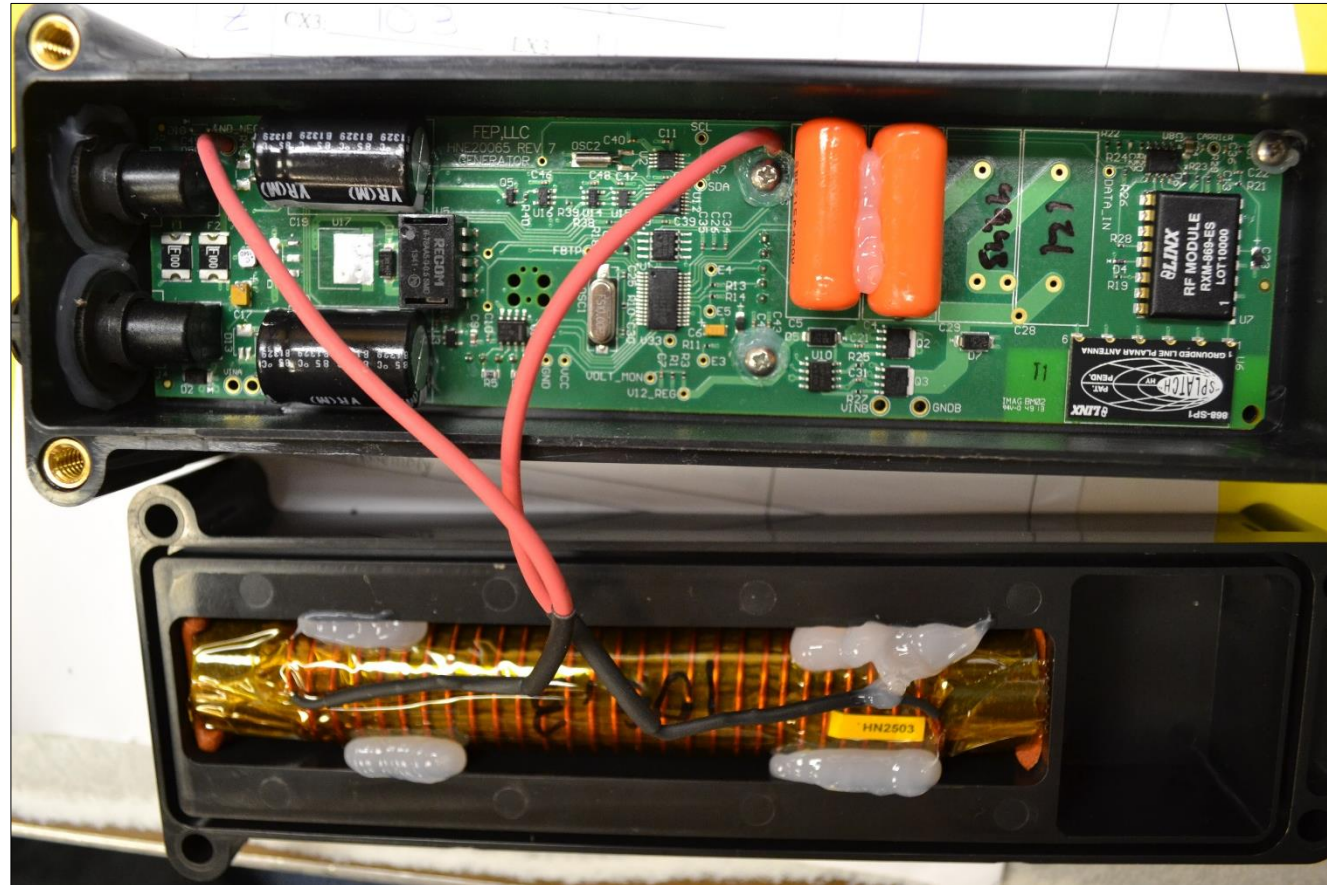
Magnetic Field Generator w/ CAM -Internal Photo Open Ferrite and Middle Housings Circuitry and Wire/Inductor
