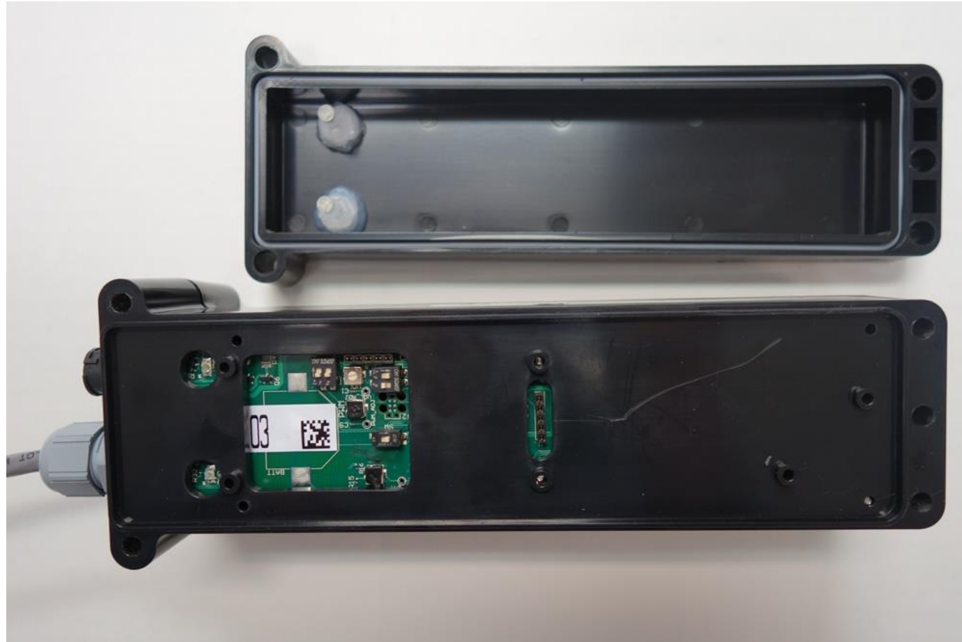
Magnetic Field Generator-Internal Photo Open Label and Middle Housings Circuitry and Wire/Ferrite Radiator
